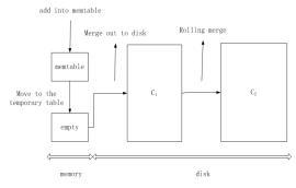
Figure 4.The process of Rolling Merge
